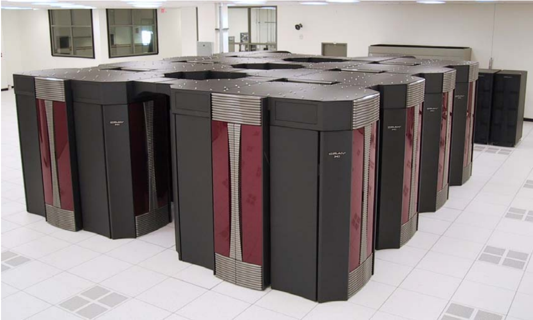
Figure 10: Elevated view of 256-MSP, 8-cabinet Cray X1 at ORNL's Center for Computational Sciences.
