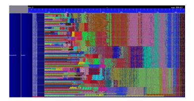
VITE is able to display millions of items. To manage such performances, an efficient data structure and a good rendering is needed. The data structure is based on sorted binary trees, as depicted in Figure 4. Thanks to these trees, any element can be accessed in logarithmic time and unneeded branches of the tree can be avoided.
